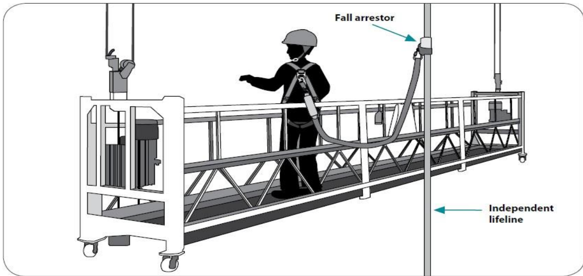
A suspended scaffold is mainly used for performing work on the sides of chimney. Workers should be protected by a personal fall arrest system with an independent vertical lifeline anchored from the top of the chimney.
