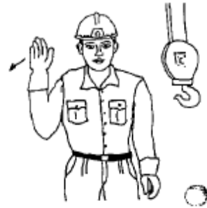
CROSS TRAVEL:-Keep the palm at the shoulder level and move it in the direction of travel required.
